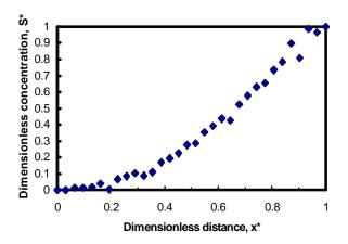
*Figure 1.* The variation of dimensionless dissolved oxygen concentration measured using microelectrode by distance through the thickness of the biofilm.
