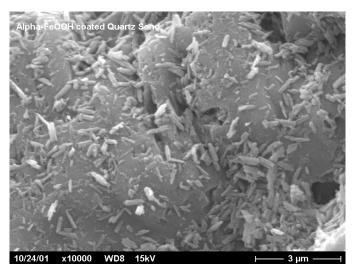
Figure 1. SEM image of a-FeOOH coated quartz sand. Goethite crystals were observed to maintain their characteristic needle-shaped structure after adsorption onto the quartz sand
