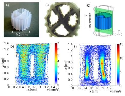
**Figure 1.** Carrier material type K1 (AnoxKaldnes, Sweden): **A)** clean carrier, **B)** cultivated carrier, **C)** setup for flow experiment. Flow velocity maps (axial plane indicated as green layer in C): **D)** clean carrier, **E)** cultivated carrier, where the black lines indicate the biofilm surface.
